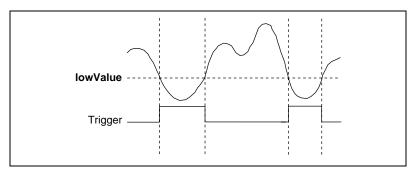
Figure 4-11. Below-Low-Level Analog Triggering Mode
