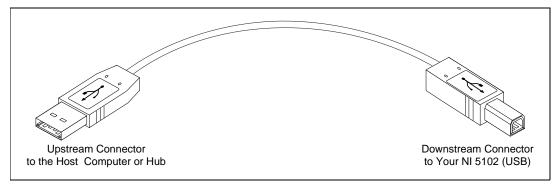
Figure 2-1. NI 5102 (USB) Upstream and Downstream Connectors
