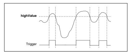
Figure 4-12. Above-High-Level Analog Triggering Mode
