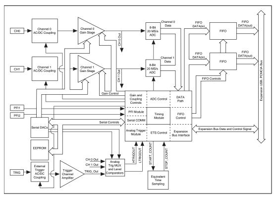
Figure 4-2 shows a block diagram of the NI 5102 (PCMCIA, USB).
