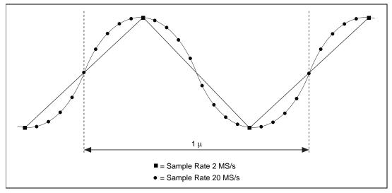
Figure 3-3. 1 MHz Sine Wave Sample
