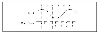
Figure 4-7. Scan Clock Delay
