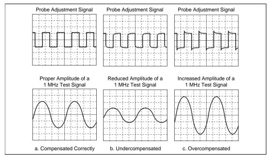
Figure 3-9. Probe Compensation Comparison
