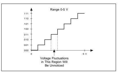
Figure 3-4. Transfer Function of a 3-Bit ADC
