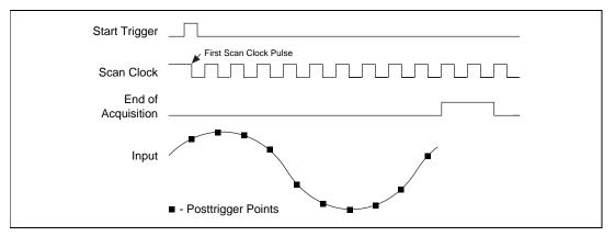
Figure 4-8. Posttrigger Acquisition
