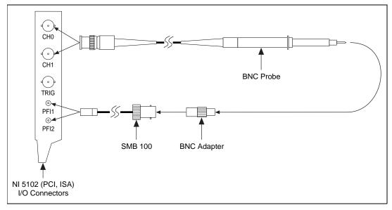
Figure 3-8. Connecting the Probe Compensation Cabling
