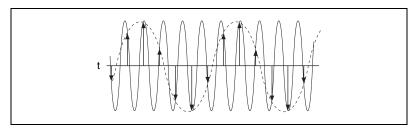
Figure 3-1. Aliased Sine Wave When Waveform is Under Sampled
