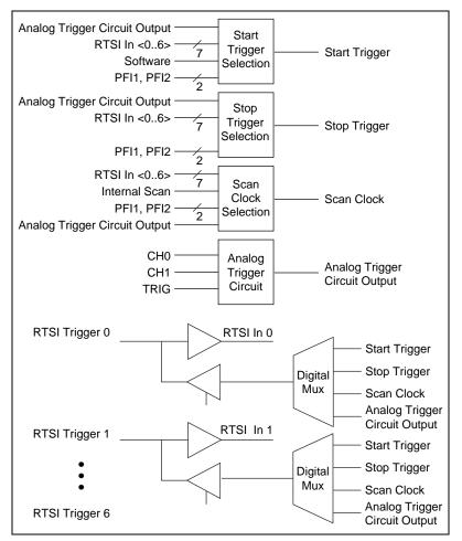
Figure 4-19. RTSI Bus Trigger Lines
