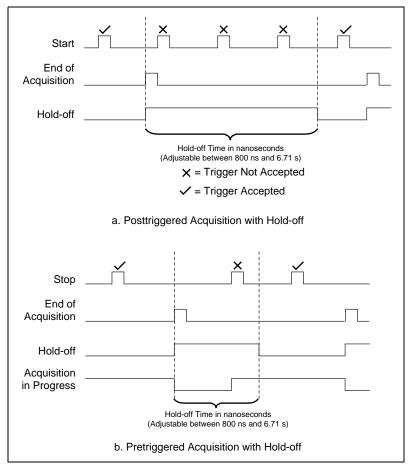
Figure 4-16. Pretrigger and Posttrigger Acquisitions with Hold-off
