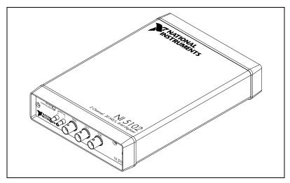
Figure 4-5. NI 5102 (USB) I/O Connectors
