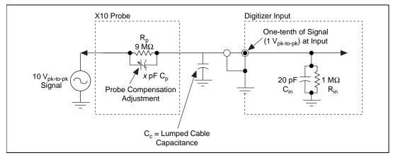
Figure 3-7. Typical X10 Probe
