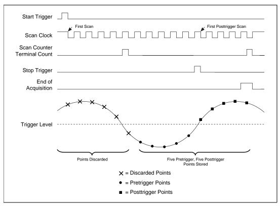
Figure 4-9. Pretrigger Acquisition
