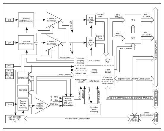
Figure 4-1. NI 5102 (PCI, PXI, ISA) Block Diagram
