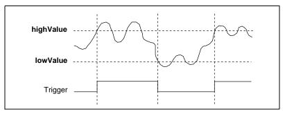
Figure 4-14. High-Hysteresis Analog Triggering Mode
