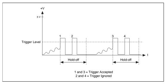
Figure 3-6. Difficult Pulse Train Signal
