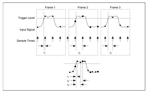
Figure 4-17. Waveform Reconstruction with RIS
