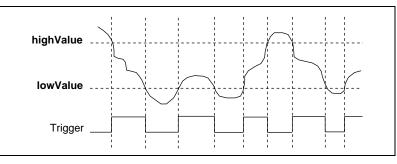
Figure 4-13. Inside-Region Analog Triggering Mode
